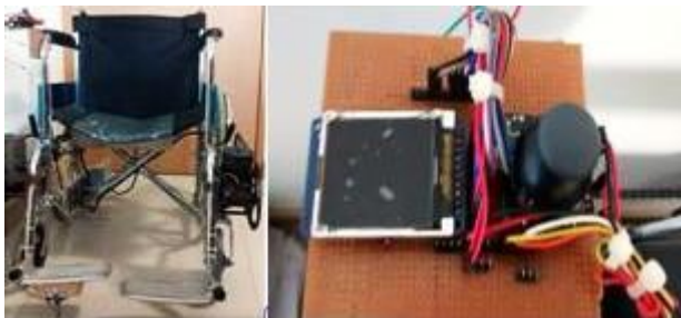
Figure 5. Mind controlled wheelchair
